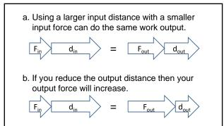
c. This means we can have a small input force create a large output force.
